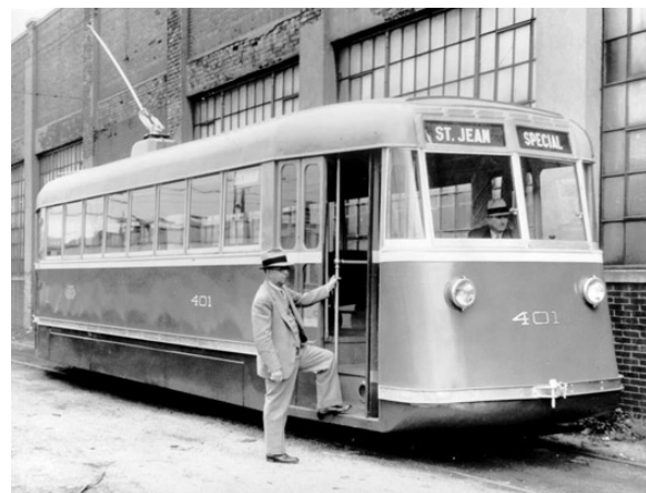
LEFT—#401 “Blue Streak” was built by the DSR in 1934 when 1 man Peter Witts replaced Birneys on the lightly traveled Woodmere line. The four 25 hp motors came from scrapped Birneys and were field tapped to give it performance well above the Peter Witts. World War II crush loads were too great to replace a Peter Witt so it was relegated to night and Sunday runs.
