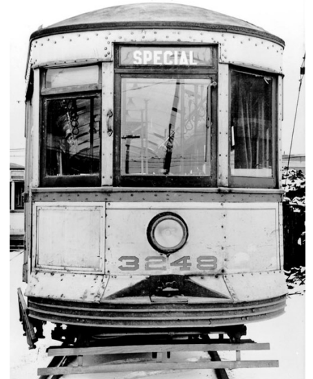
LEFT—#3248 in 1940 after rebuild by the DSR. The new front end probably came from a scrapped Peter Witt that was gutted by fire. The Brill-77 trucks were rebuilt and covered with sheet metal to reduce and contain track noise. Performance was enhanced by replacing 35hp motors with 50 hp motors.
